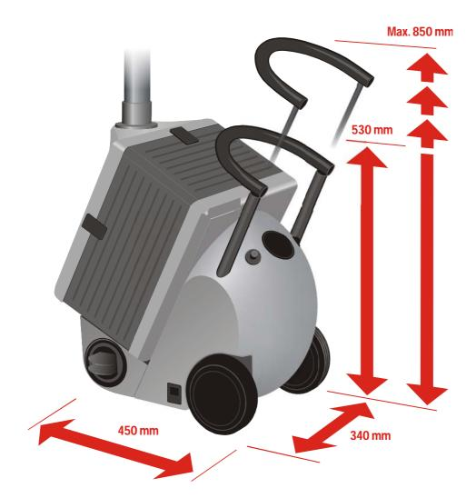
max. air flow: max. vacuum: constant air flow: electrical connection: input power: dimension: weight: noise level: 170 m<sup>3</sup>/h 2,800 Pa 80 m<sup>3</sup>/h at 1,400 Pa 230 V/50 Hz 150 W 450 x 340 x 530 mm 18 kg 49 db (A)
